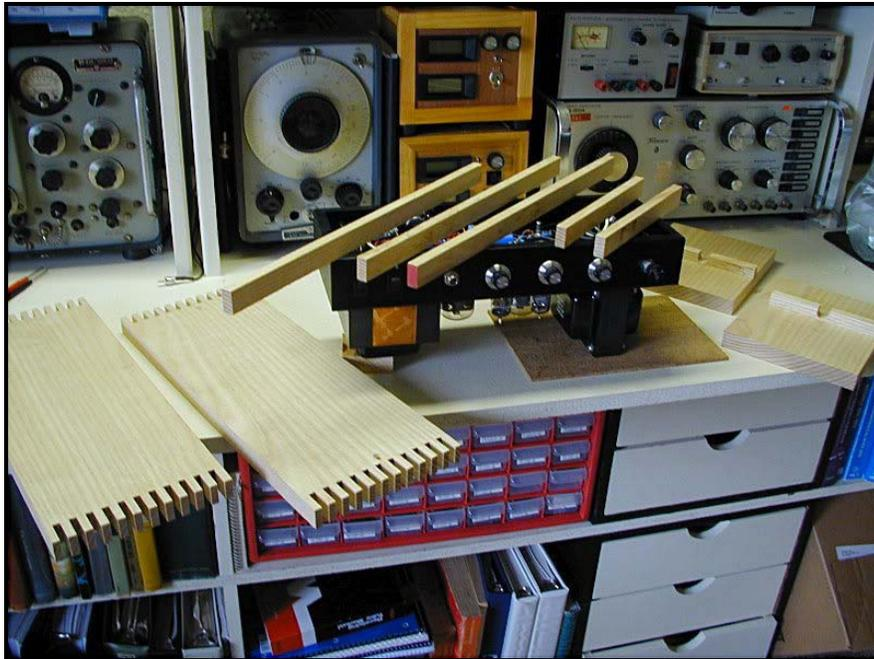
After all joints have been machined, the enclosure is assembled, two pieces at a time. Glue is brushed into the finger joints and the two parts are tapped together using a soft-faced mallet. The pieces are clamped into position while the glue is curing after first assuring that they are square to one another by checking with a carpenter's or machinist's square.
