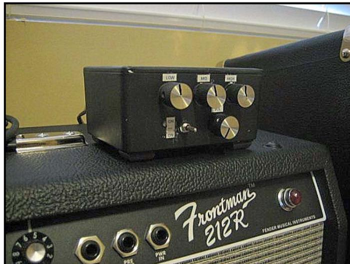
A preamplifier like this one is a useful addition to one's collection of cables, instruments, microphones and tools and can be built compactly enough to fit in a guitar case (or in the bottom of a combo amplifier). Note that the output is high impedance, however, and therefore long cables from the preamplifier are not recommended.
