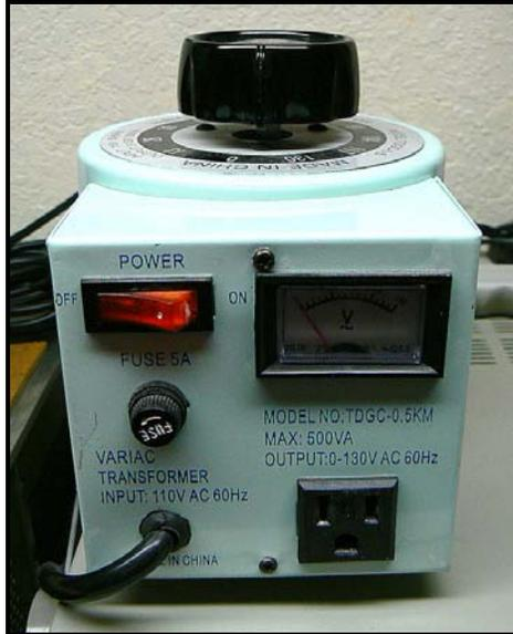
Observe that a line cord is required to connect the autotransformer to the power supply. This particular model is rated at 500 VA (volt-amperes). To be safe, it's normal to de-rate these devices by 50%, therefore the operating conditions shouldn't exceed 250 VA at the input:
