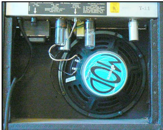
After replacing speaker and transformer, a listening test left me desiring a more balanced response - the Champ always lacked bass. I measured the frequency response of the new configuration then experimented with partly covering the back of the enclosure until I arrived at this variation, which has a satisfying amount of bass and midrange. One of these days, I'll get around to painting that piece of cedar.
