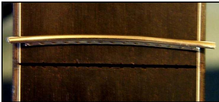
The "tang" of the fret wire (the portion of the fret that is forced into the fret slot of the fingerboard) must be removed from the fret at each end. In the above photo, a close look reveals that the tang has been clipped and filed or otherwise
