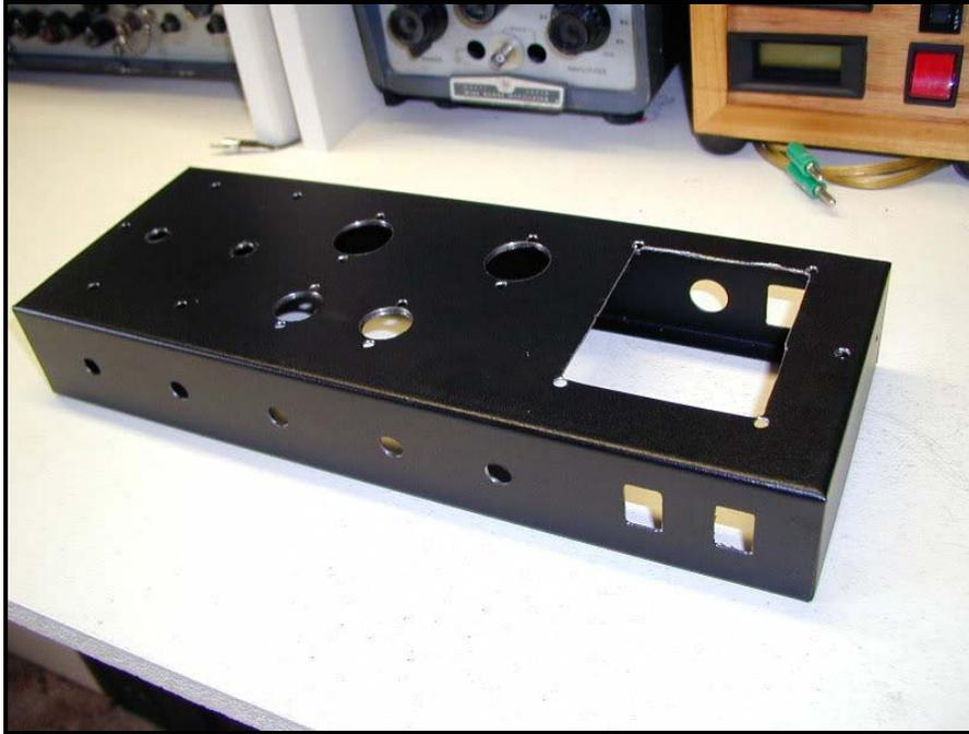
All of the work performed on this chassis can be accomplished in an afternoon with a drill press, the tools mentioned above and a "nibbler". It's even possible to do this work with a hand drill (drilling a sequence of holes that are almost tangent to one another, breaking out the waste material and then filing edges smooth) and I have often done so, when more suitable tools were lacking.
